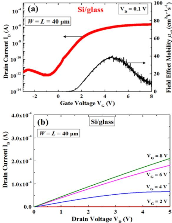
**Figure 3.** (a) Transfer and (b) output characteristics of a fabricated poly-Si TFT for Si/glass structure with  $W = L = 40$   $\mu\text{m}$
