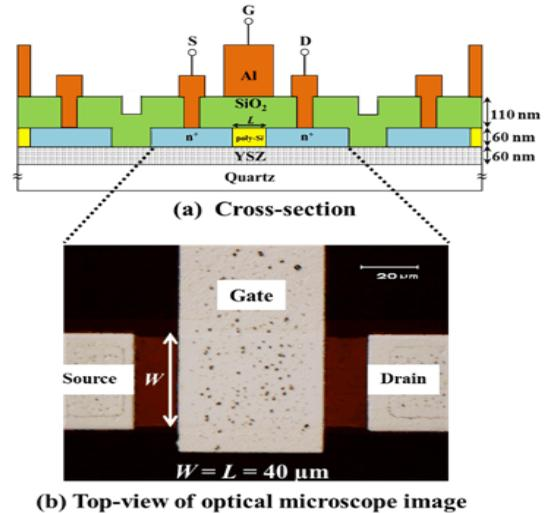
**Figure 2.** (a) Cross-sectional schematic illustration and (b) top-view of optical microscope image of a fabricated poly-Si TFT
