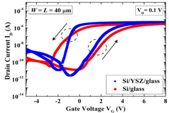
**Figure 5.** Hysteresis phenomenon occurring in the transfer characteristics of fabricated poly-Si TFTs with  $W = L = 40 \mu\text{m}$  at  $V_D = 0.1$  V for the two structures of the Si/glass and Si/YSZ/glass
