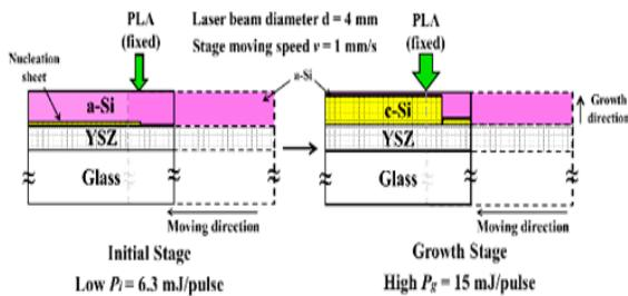
**Figure 1.** Schematic illustration for crystallization by the two-step PLA method together with irradiation conditions
