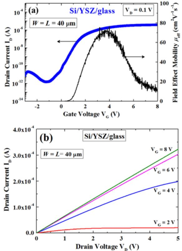
**Figure 4.** (a) Transfer and (b) output characteristics of a fabricated poly-Si TFT for Si/YSZ/glass structure with  $W = L = 40$   $\mu\text{m}$
